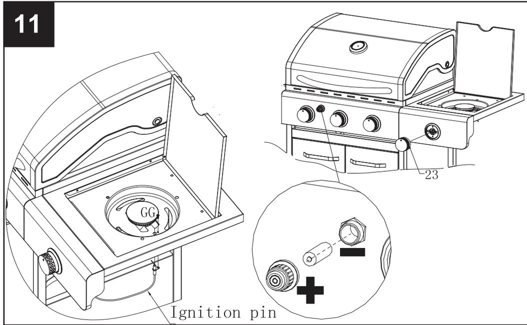
Assemble the side burner rack(19) to the side burner table, put the warming rack(16) ,cooking grills(17),flame tamer (18) into the body.
