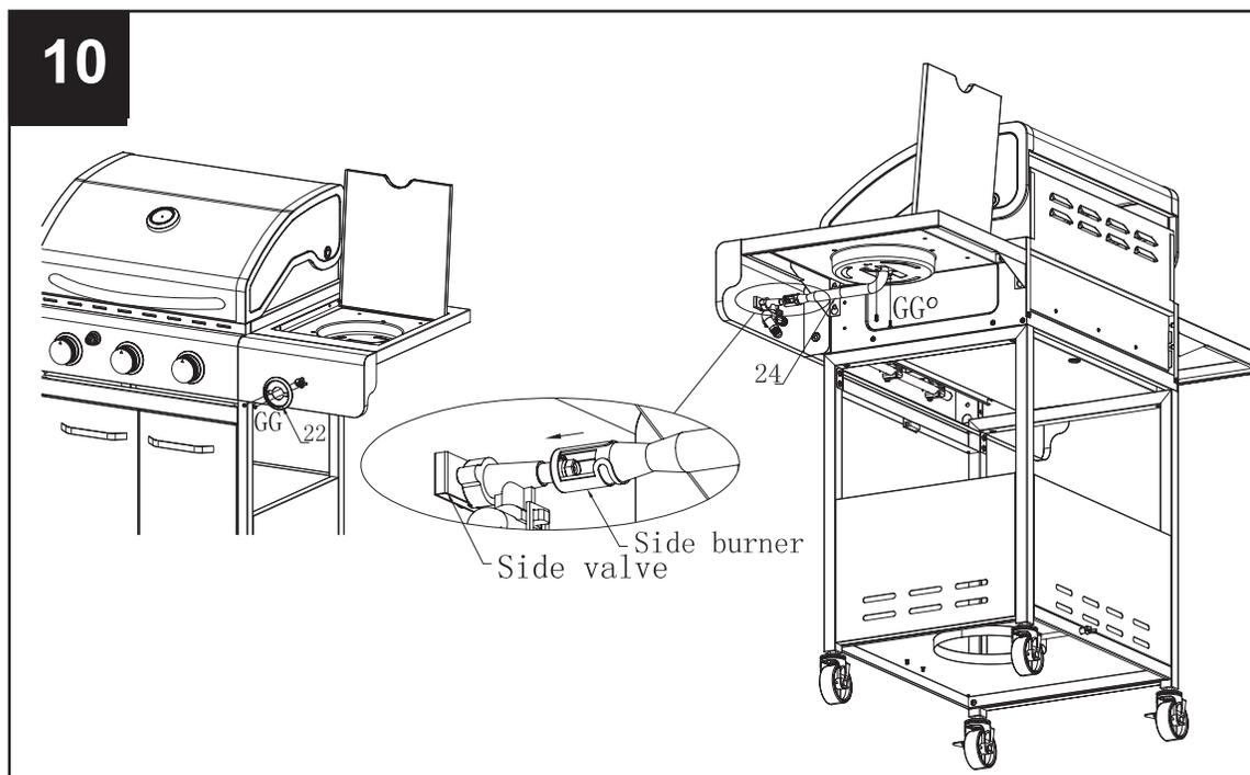
**⚠ WARNING: IT IS VERY IMPORTANT TO CHECK AND ENSURE THAT EACH AND EVERY BURNER IS FULLY ENGAGED WITH THE ADJACENT VALVE ORIFICE BEFORE COMPLETING STEP 10. FAILURE TO DO SO MAY RESULT IN FIRE OR EXPLOSION, POSSIBLY CAUSING SERIOUS INJURY OR DEATH. REFER TO MAINTENANCE SECTION INSTRUCTIONS TO PROPERLY CHECK THE ENGAGEMENT.**
