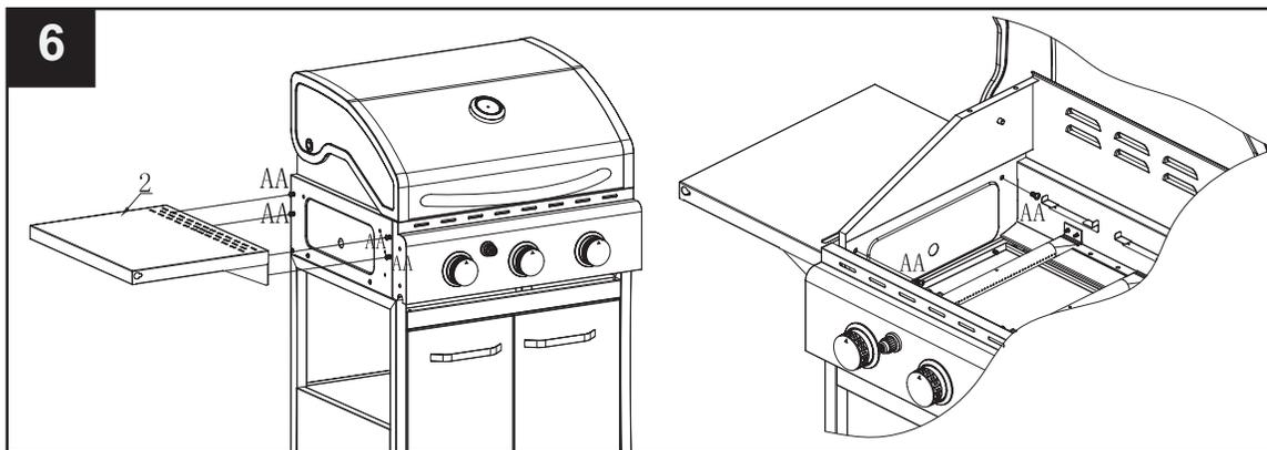
First Assemble the Bottle opener (7) to the left front panel (3) using M4x10mm bolts(JJ). Assemble the M6x12mm to the the left front panel, reserve a distance of 5mm. Then fix the left front panel (3) to the body using M5x10 bolts (BB).
