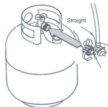
5. Hand-tighten the coupling nut ↻ clockwise until it comes to a full stop. Firmly tighten by hand only. Do not use tools.
